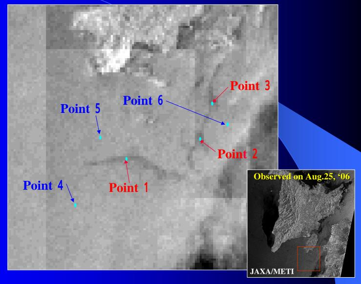
The sampling points are selected in the area detected as an spilled area : Point 1  $\sim$  3 The sampling points are selected in the normal sea surface area : Point 4  $\sim$  6
