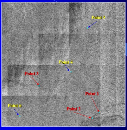
The sampling points are selected in the area detected as an spilled area : Point  $1 \sim 3$
